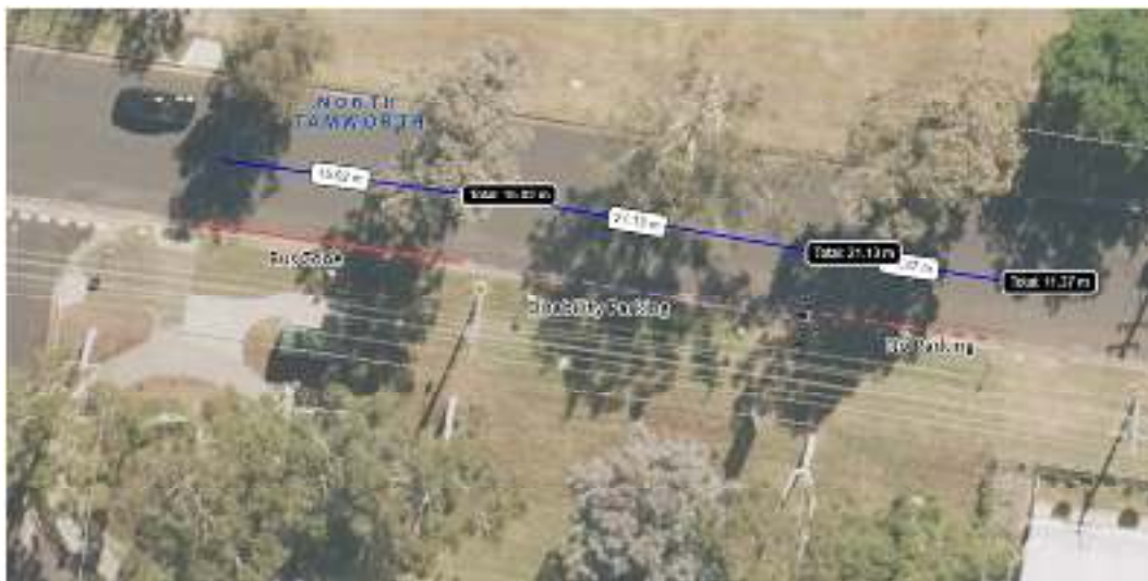
Image 5: Proposed lay out of bus zone, disabled parking and no parking on Johnston Street
